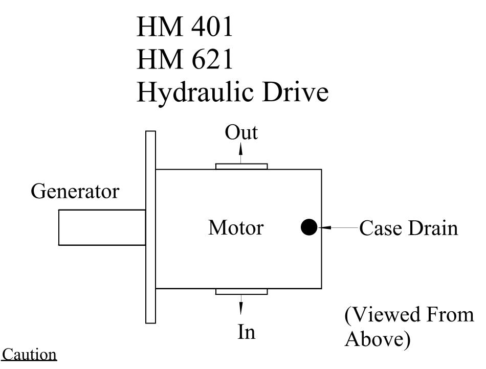
Do not allow generator to exceed 3800 RPM
